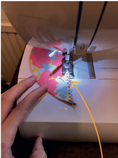
Brim opening closed with a 0.5cm seam allowance
