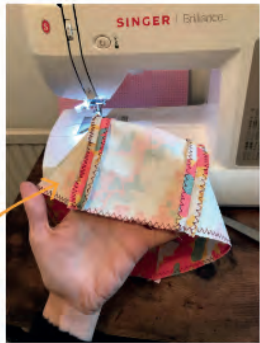
Seam allowance pressed open along crown
