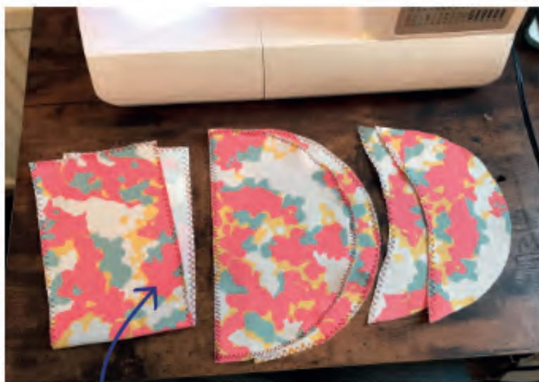
Edges finished with a zig zag stitch
